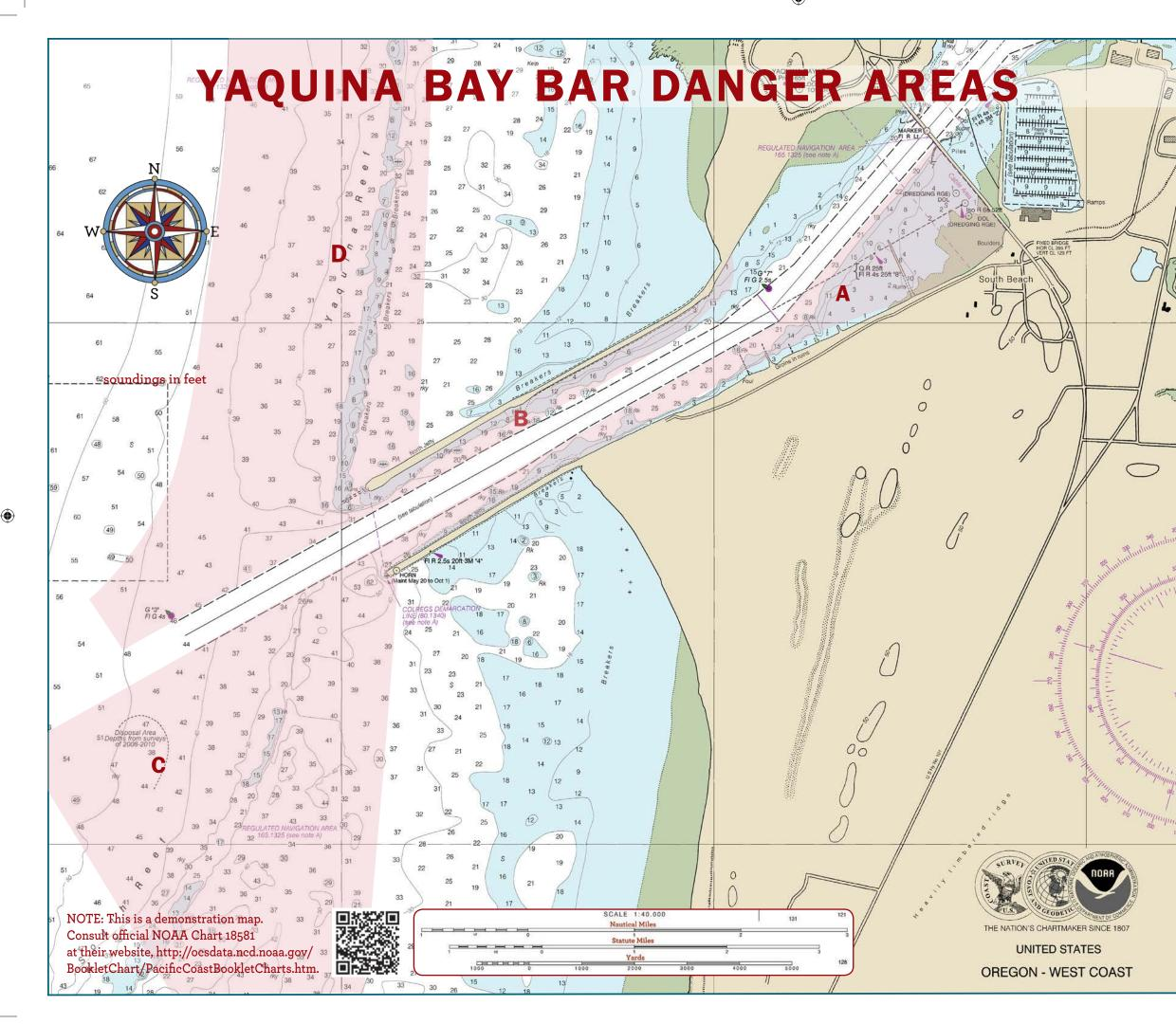
A. South jetty. There are submerged rocks along the length of the jetty; do not hug the jetty on either side. Boaters should remain in the channel entering and leaving the river so that if their engines fail, they will have time to anchor before the current or wind sweeps them into the rocks.
